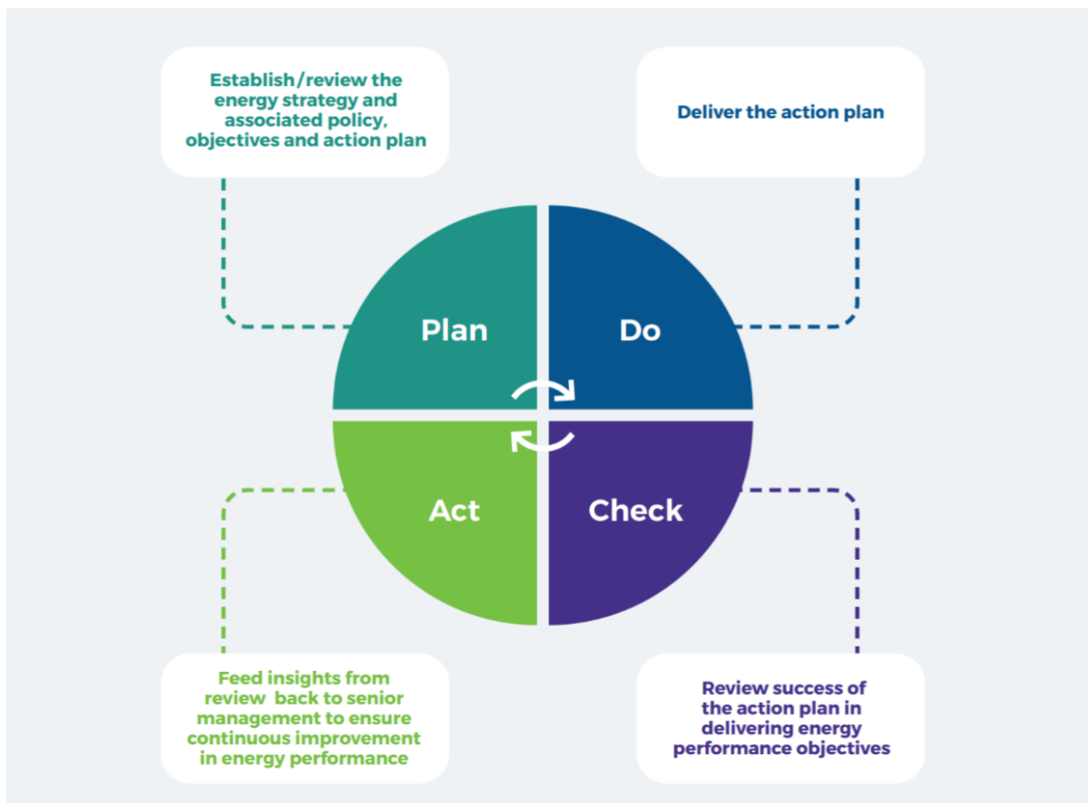
Figure 3 – An illustration of the Plan-Do-Check-Act approach in relation to EnMS
